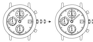
3.Pull out the crown to the second click when the second hand is at the 12 o'clock position. It will stop on the spot and advance the hour and minute hands by turning the crown. (Check that AM/PM is set correctly.)
