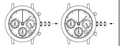
3.Pull out the crown to the second click when the second hand is at the 12 o'clock position. It will stop on the spot and advance the hour and minute hands by turning the crown. (Check that 24 hour hand is set correctly.)
