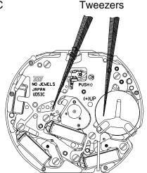
2) When the battery replaced with a new one, the time information stored in the built-in IC and the time indicated by the stopwatch hands do not correspond with each other. Reset the stopwatch hands to "0" position following the procedure below. If the stopwatch hands should move improperly, also follow the same procedure.
